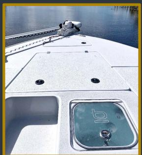
Bonefish boats are designed using a semi-monocoque technique to promote strength and rigidity, and are constructed from premium uv-resistant gelcoat, epoxy vinyl ester resin and high-density fiber-reinforced transom board.
